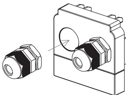
1-4. Screw the end cap which is closed to the wire input to the trunking rail.
