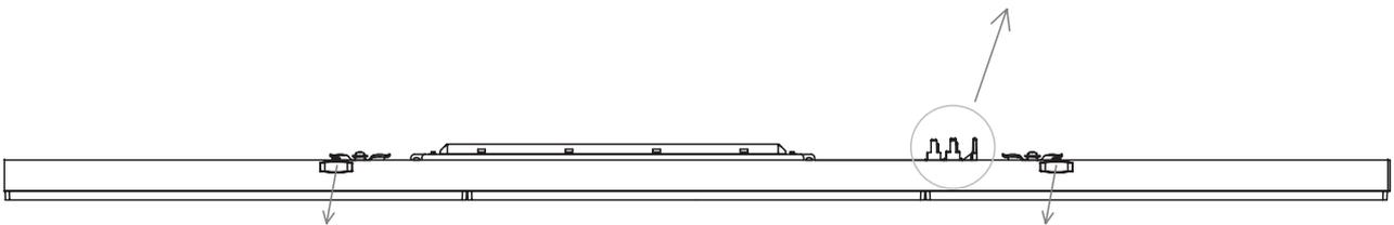
3. Match electronic connector in the luminaire to the socket in the trunking rail while locking.
