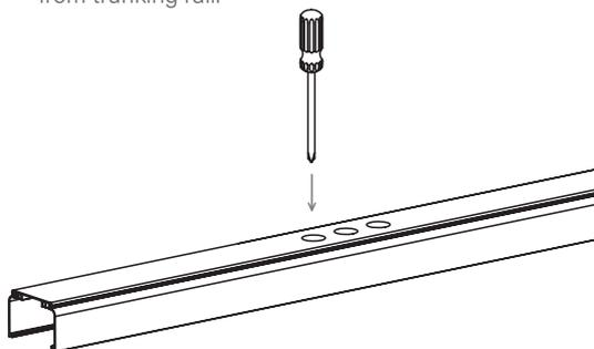
Note: 2 holes for 5/7 wires, 3 holes for 11 wires.
