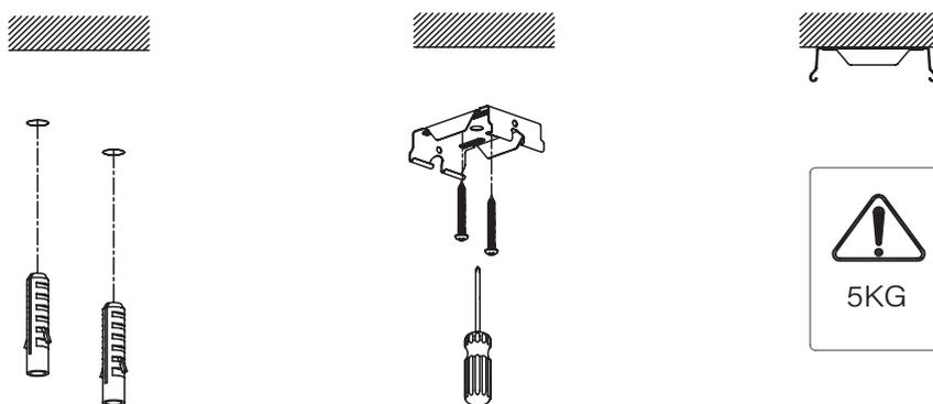
Note: The distance between two surface mounted kits is adjustable, 3m maximum.
