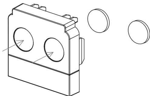
Note: 1 holes for 5 wires, 2 holes for 7/11 wires.
