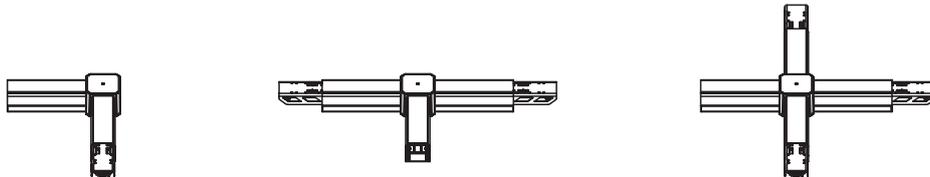
4-2. Remove connector in the trunking rail firstly, roll over wires back to the rail, screw end cap.
