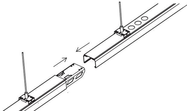
2. Pull out the lock bar of luminaire.
