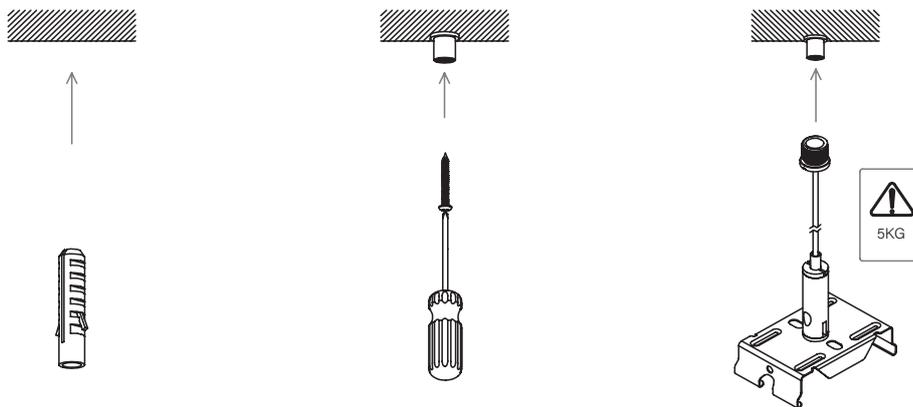
Note: The distance between two suspension kits is adjustable, 3 m maximum.
