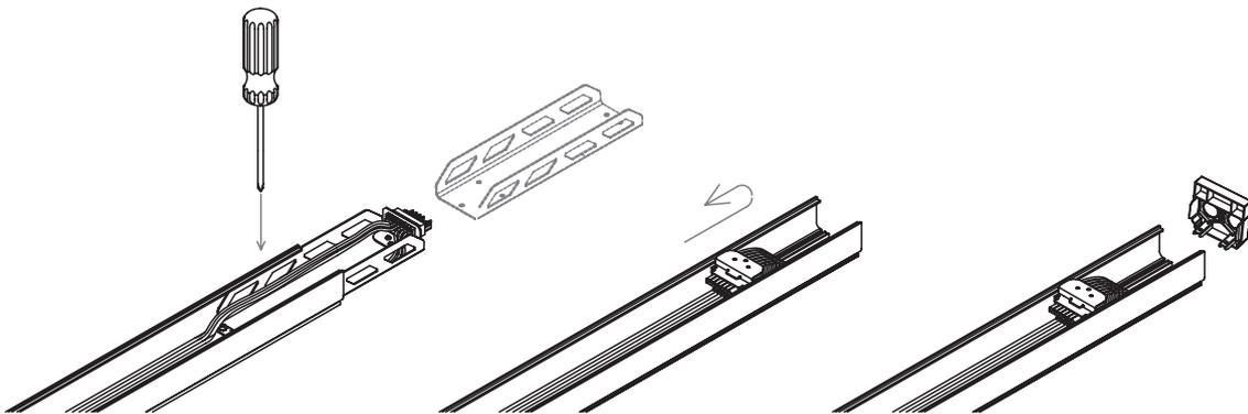
Note: Optional closing: "—" type end box is to make it easier to close the end of linear system. Push it to the trunking rail to cover the connector, no need to remove it.
