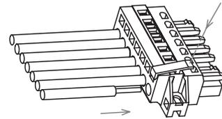
Note: Using wired tool to help to connect wires, please remove the tool after usage.
