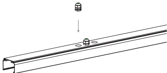
1-4. Screw the end cap which is closed to the wire input to the trunking rail.
