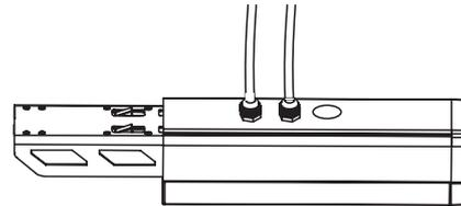
Note: "—" type feed-in node connector is optional to input wire easily. Input wire from the back of "—" type feed-in node connector on hand firstly, and then push it to the linear system directly.
