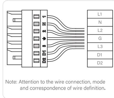
2-2. Join terminal block (CCLA-ITS) to male in the trunking rail.
